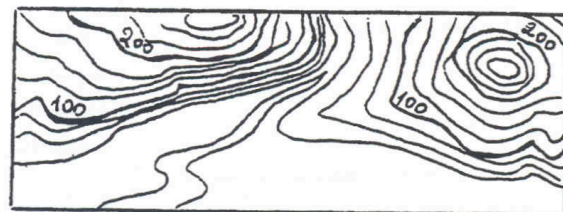
Figure 2 illustrates how contour lines illustrate the same location on a 2 dimensional map.
